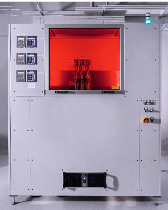
Fig. 1 • System for Multi Material Jetting of high-performance components with combined properties or functions. (All pictures Fraunhofer IKTS)
