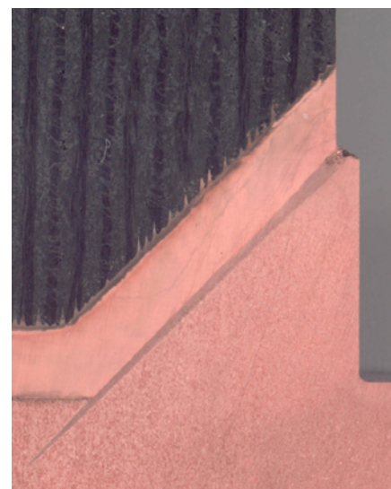
Lowest heat penetration thanks to a particularly narrow weld seam. (Photo: PTR Strahltechnik)
