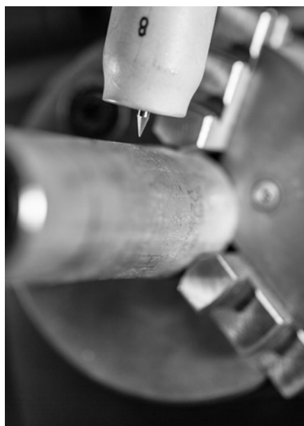
Orbital welding is frequently used in the manufacturing trade, for applications ranging from installing cooling and heating pipes in dairies to welding fuel pipes in the aerospace sector. (Photos: Gesellschaft für Wolfram Industrie GmbH)
