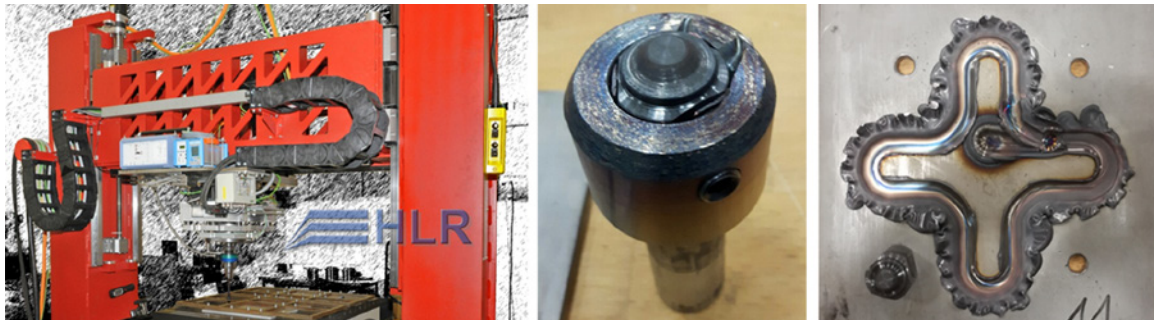
Fig. 5 • Experimental set-up for test under realistic conditions with FSW-machine from HLR Systems, Germany (left), tool holder including \text{Si}_3\text{N}_4 -tool (middle), test route (right).
