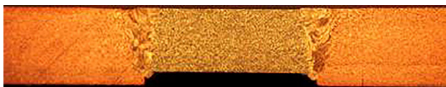
Microsection of a tri-band weld (copper–copper manganese–copper)
