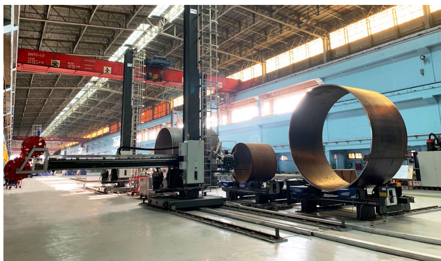
The "Pema" production automation lines are designed to manufacture pin piles for offshore jacket foundations.
