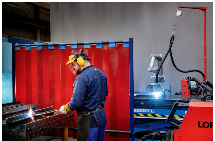
While the Lorch Cobot accurately draws the weld seams set for a repeat part, the welder can already prepare the next serial part. (Photo: Lorch)
