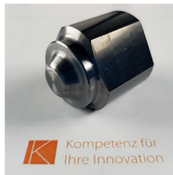
Fig. 9 • First produced FSW tool made of \text{WC-ZrO}_2 .
