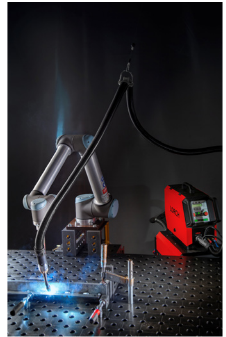
Tidy welding bench and swift integration: A key advantage of Lorch's collaborative robot welding is the reduced effort when using fixtures. (Photo: Lorch)
