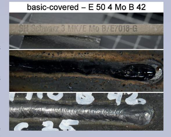
Basic-covered stick electrodes are suitable for welding in all positions, except the vertical-down position. Basic stick electrodes which are especially suitable for welding in the vertical-down position have a covering with a particular composition.
