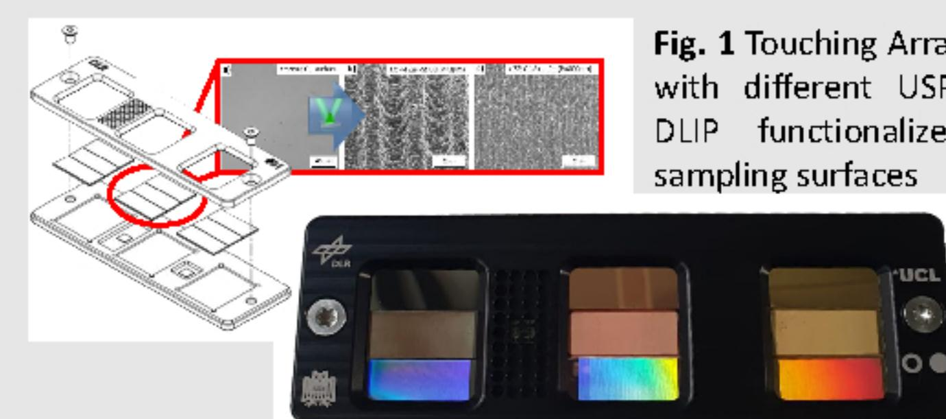
Fig. 1 Touching Array with different USP-DLIP functionalized sampling surfaces
